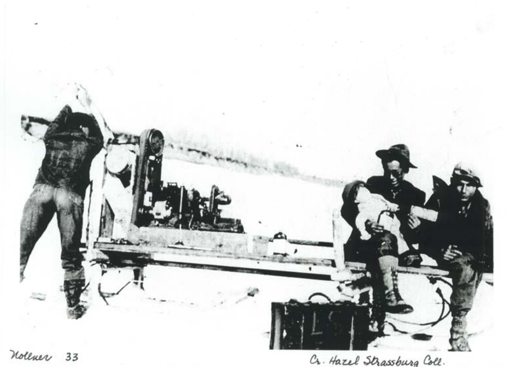
Galena's first "snow machine" made from two bobsleds with an inboard motor engine. According to Hazel Strassburg, it didn't steer too well. All the kids would run after it hoping for a ride, but usually ended up helping to tow it back. Left to Right) Lincoln Antoski, Lincoln Stockman, with Josephine Robert's doll, and Alfred Demoski. Photo taken near Galena in the early 1930's.
